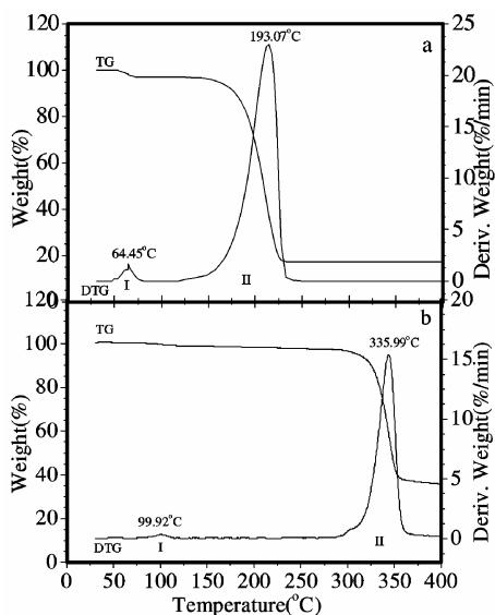
**Figure 1.** TG-DTG curves of thermal decomposition ( $\beta = 10^\circ\text{C}/\text{min}$ ). (a)  $\text{LiPF}_6$ , (b) LiBOB.
