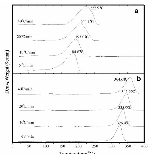
**Figure 2.**  $\theta_m$  of the second decomposition step in DTG curve with various  $\beta$ . (a)  $\text{LiPF}_6$ , (b) LiBOB.
