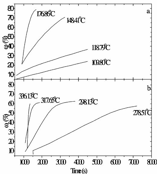
**Figure 3.**  $\omega$  at the time of  $t$  with different  $\theta_C$ . (a) LiPF<sub>6</sub>, (b) LiBOB.
